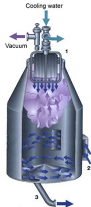
Fig. 6.6.4 Flow of milk and air in the vacuum deaerator with built-in condenser.
